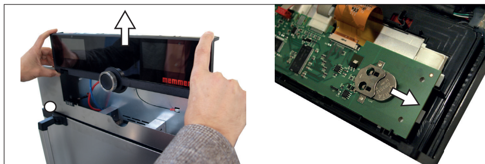
Fig. 41 Removing the lithium battery
