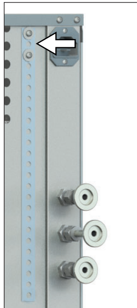
Fig. 14 Install tilt protection on the backside
