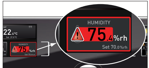
Fig. 23 Humidity monitoring triggered
