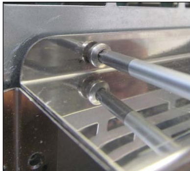
Fig. 5 Screw the exhaust air unit tight
