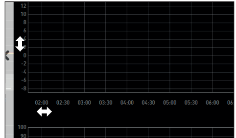
Fig. 11 Scaling the time or value axis by scrolling as soon as the mouse cursor turns into a double arrow
